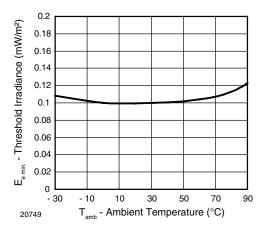
Fig. 10 - Sensitivity vs. Ambient Temperature
