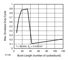
Fig. 9 - Maximal Envelope Duty Cycle vs. Burst Length
