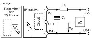
$\rm R_1$  and  $\rm C_1$  are recommended for protection against EOS. Components should be in the range of 33  $\Omega$  <  $\rm R_1$  < 1 k $\Omega,$  C\_1 > 0.1  $\mu F.$
