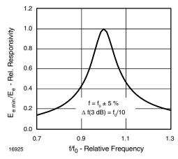
Fig. 5 - Frequency Dependence of Responsivity
