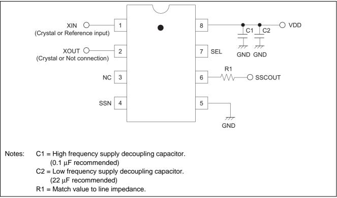
Figure 2 Recommended circuit configuration
