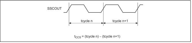
Figure 1 Cycle to cycle jitter
