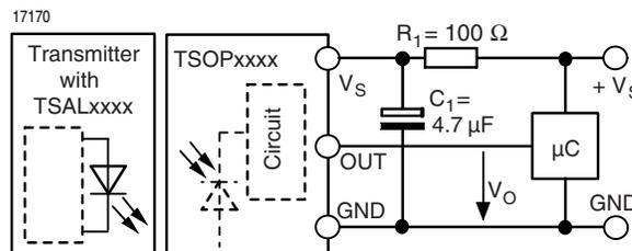
$R_1$  and  $C_1$  recommended to suppress power supply disturbances. The output voltage should not be hold continuously at a voltage below  $V_O = 2.0$  V by the external circuit.
