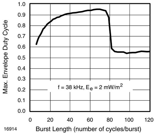
Fig. 9 - Maximum Envelope Duty Cycle vs. Burst Length
