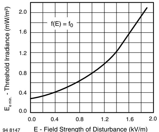
Fig. 8 - Sensitivity vs. Electric Field Disturbances
