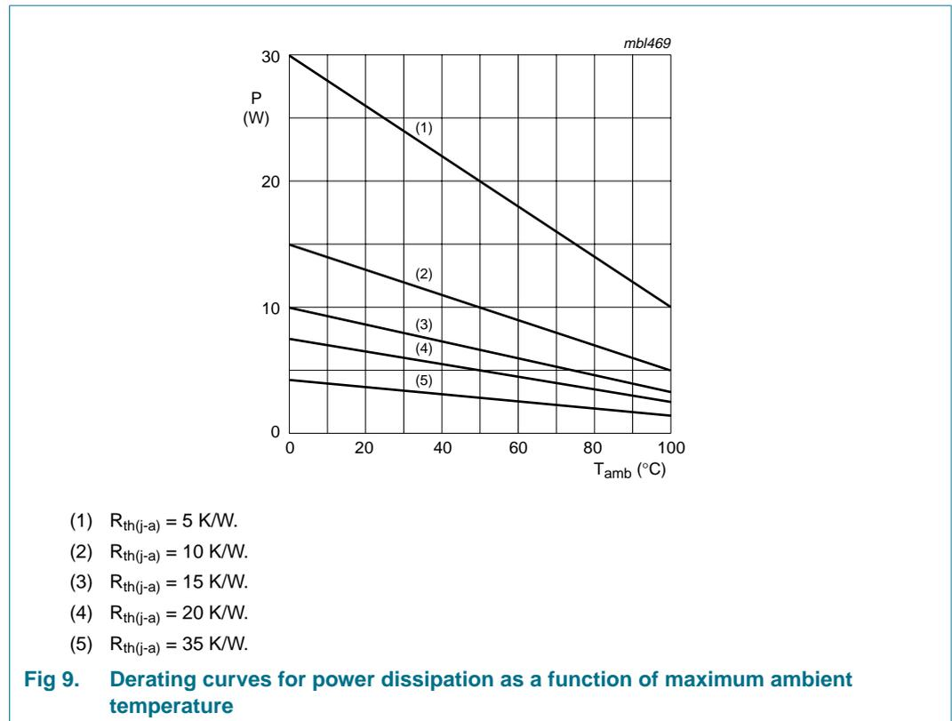
In the following example, a heatsink calculation is made for an 8 Ω BTL application with a ±30 V supply:
