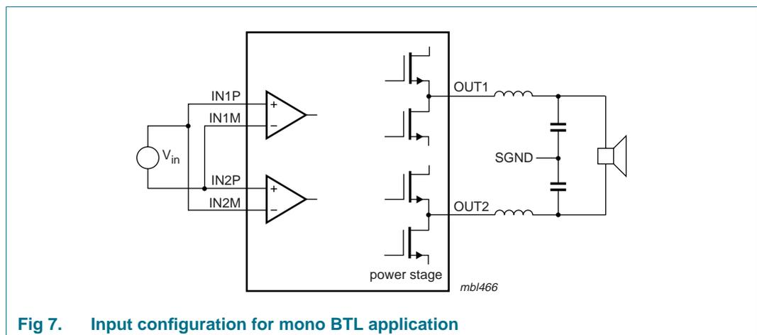
**Fig 7. Input configuration for mono BTL application**
