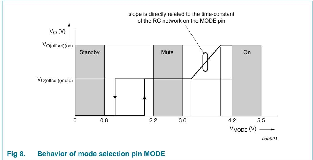
Fig 8. Behavior of mode selection pin MODE
