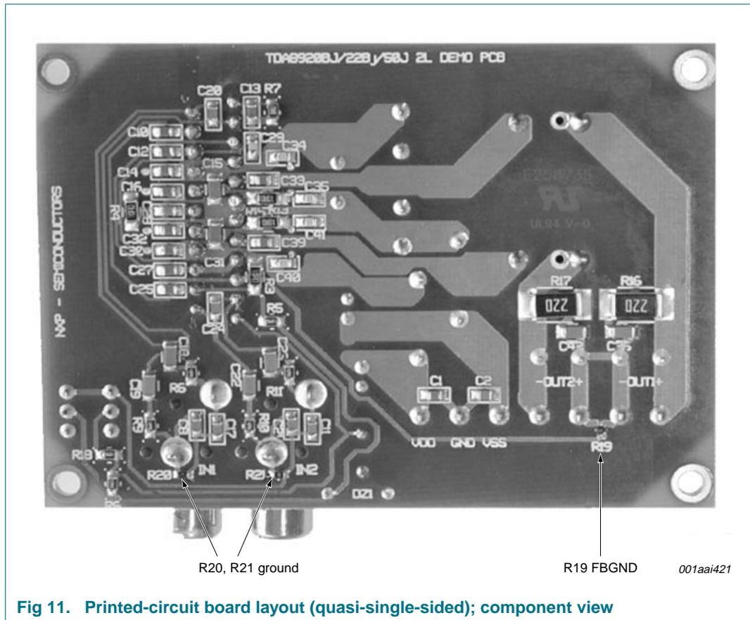
Fig 11. Printed-circuit board layout (quasi-single-sided); component view
