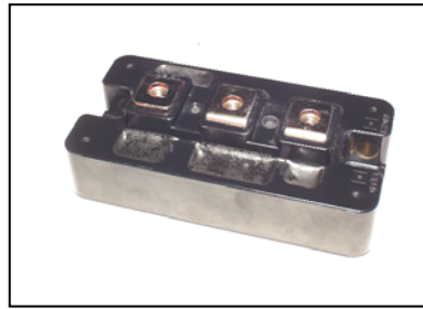
QIQ0630003 Low side Chopper IGBT Module 300 Amperes / 600 Volts
