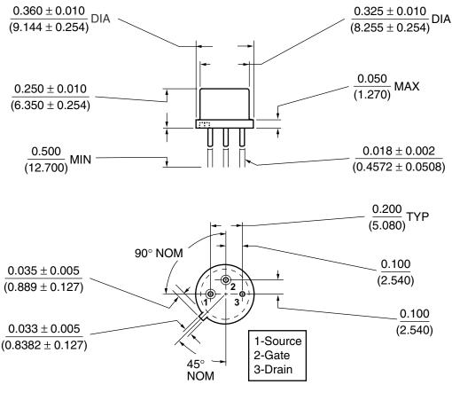
$Measurement Legend = \frac{Dimensions in Inches}{(Dimensions in Millimeters)}$
