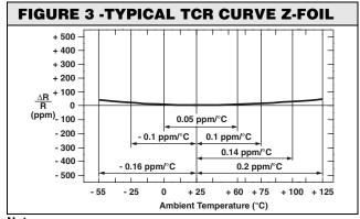
The TCR values for < 100  $\Omega$  are influenced by the termination composition and result in deviation from this curve.
