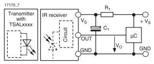
The external components R<sub>1</sub> and C<sub>1</sub> are optional to improve the robustnes against electrical overstress (typical values are R<sub>1</sub> = 100  $\Omega$ , C<sub>1</sub> = 0.1  $\mu$ F). The output voltage V<sub>o</sub> should not be pulled down to a level below 1 V by the external circuit.
