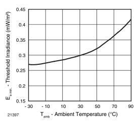
Fig. 10 - Sensitivity vs. Ambient Temperature
