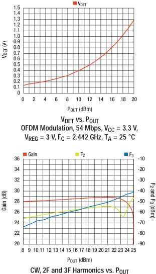
CW, 2F and 3F Harmonics vs.  $P_{OUT}$ V<sub>CC</sub> = 3.3 V, V<sub>REG</sub> = 3 V, F<sub>C</sub> = 2.442 GHz, T<sub>A</sub> = 25 °C
