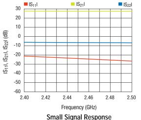
Conditions:  $V_{CC} = 3.3 \text{ V}$ ,  $V_{REG} = 3 \text{ V}$ ,  $T_A = 25 \text{ °C}$
