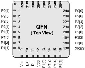
Table 2. 32-Pin Part Pinout (QFN)
