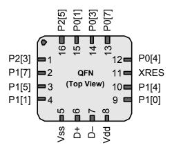
Table 1. 16-Pin Part Pinout (QFN)
