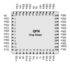
Table 3. 48-Pin Part Pinout (QFN)
