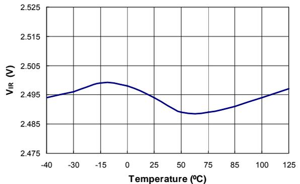
Figure 11. Reference Voltage (V<sub>IR</sub>) vs. Temperature
