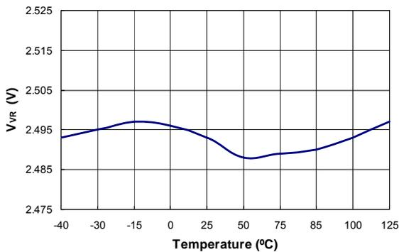
Figure 10. Reference Voltage (V<sub>VR</sub>) vs. Temperature
