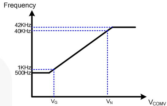
Figure 25. Green Mode Frequency vs. V<sub>COMV</sub>
