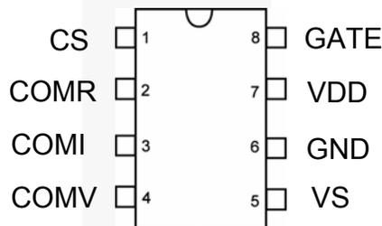
Figure 5. Pin Configuration
