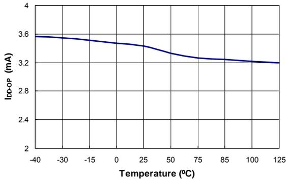
Figure 8. Operating Current (I<sub>DD-OP</sub>) vs. Temperature
