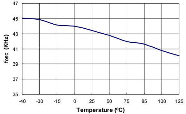
Figure 9. Center Frequency (f<sub>osc</sub>) vs. Temperature
