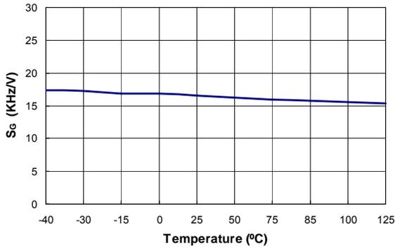
Figure 14. Green Mode Frequency Decreasing Rate (S<sub>G</sub>) vs. Temperature
