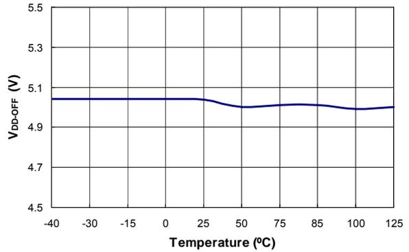
Figure 7. Turn-off Threshold Voltage (V<sub>DD-OFF</sub>) vs. Temperature
