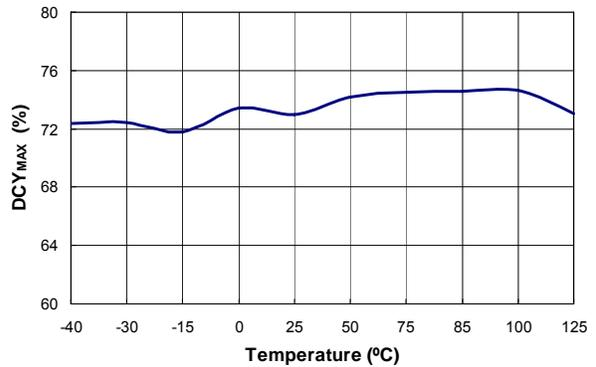
**Figure 23. Maximum Duty Cycle ( $DCY_{MAX}$ ) vs. Temperature**
