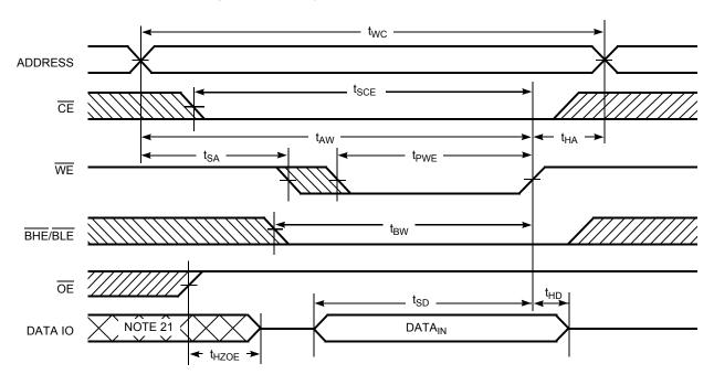
Figure 8. Write Cycle 2: CE Controlled [15, 19, 20]
