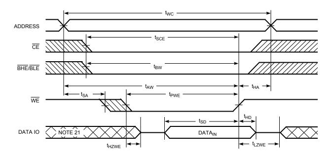
Figure 10. Write Cycle 4: BHE/BLE Controlled, OE LOW [20]
