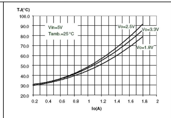
**Figure 8. Junction temperature vs output current**
