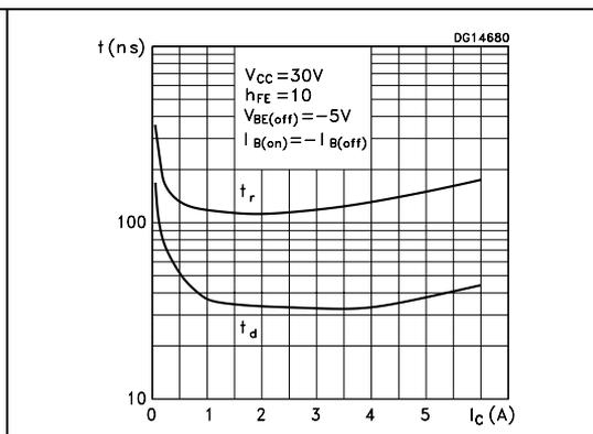
**Figure 8. Switching time resistive load** **Figure 9. Collector-base and collector-emitter capacitance**
