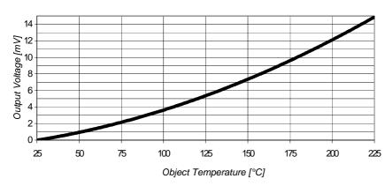
Conditions: Distance Thermopile/Black Body 5 cm, emissivity= 1, surrounding temperature 25°C
