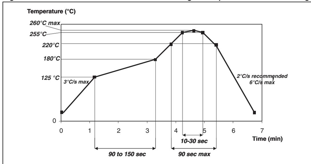
Note: Minimize air convection currents in the reflow oven to avoid component movement.
