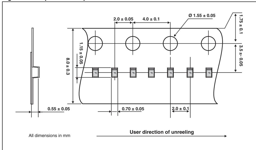
Note: Product marking may be rotated by 90° for assembly plant differentiation. In no case should this product marking be used to orient the component for its placement on a PCB. Only pin 1 mark is to be used for this purpose.
