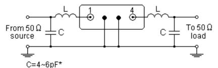
L=2 turns of 0.5mm insulated Copper, 3.0mm ID
