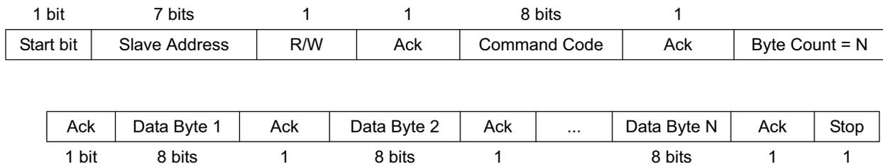
**Figure 7. An Example of a Block Write<sup>[6]</sup>**
