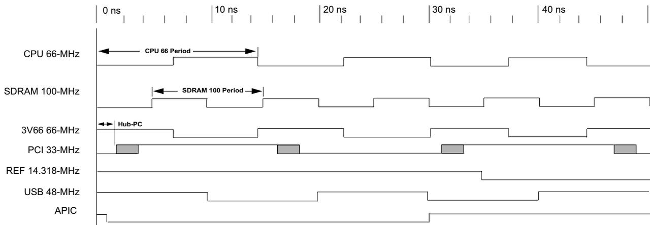
**Figure 2. Group Offset Waveforms (66.8 CPU Clock, 100.2 SDRAM Clock)**
