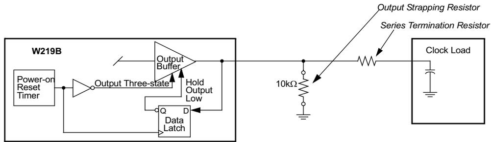
**Figure 1. Input Logic Selection Through Resistor Load Option**
