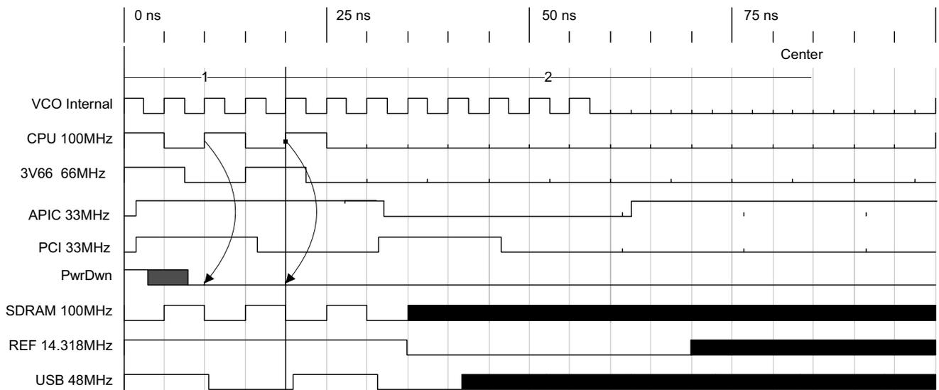
**Figure 4. PWRDWN# Timing Diagram**<sup>[2, 3, 4, 5]</sup>
