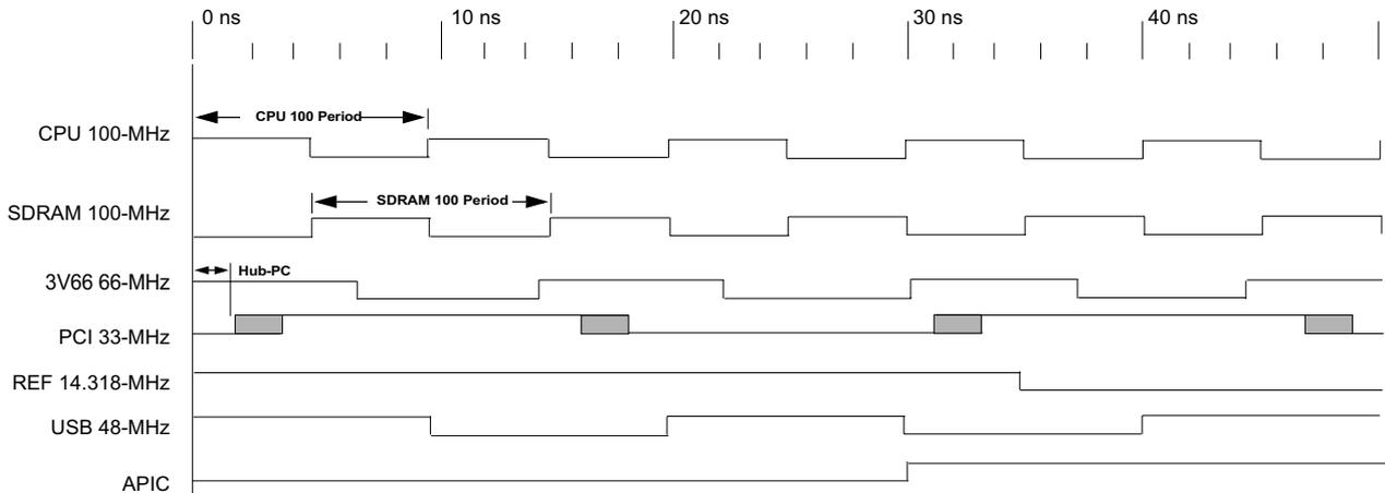
**Figure 3. Group Offset Waveforms (100.2 CPU Clock, 100.2 SDRAM Clock)**
