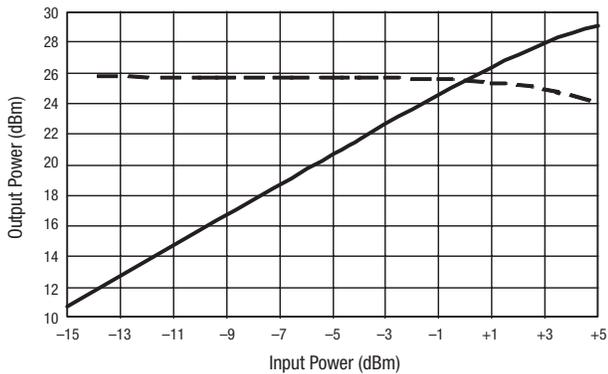
**Figure 3. Typical P<sub>OUT</sub> and Gain vs P<sub>IN</sub> @ 2.442 GHz**
