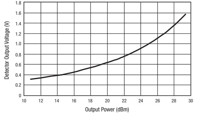
**Figure 8. Detector Output Voltage vs RF Output Power**
