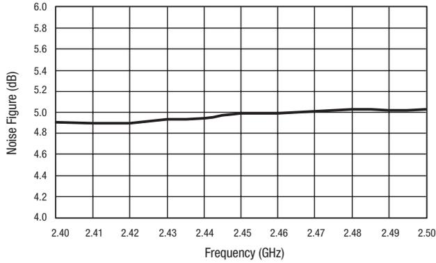
**Figure 5. Typical Noise Figure Performance vs Frequency**
