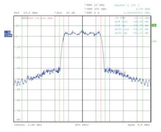
$\begin{array}{l} \mbox{SKY65112 IS-95, F} = 1960 \mbox{ MHz} \\ \mbox{V}_{CC} = 5 \mbox{ V, V}_{REF} = 5 \mbox{ V, I}_{CCQ} = 260 \mbox{ mA,} \\ \mbox{Clock freq 9.8304 MHz} \end{array}$
