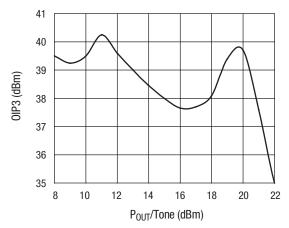
SKY65112 OIP3,  $V_{CC} = 5$  V,  $V_{REF} = 5$  V,  $I_{CCO} = 260$  mA, F = 940 MHz, Tone Spacing = 1 MHz
