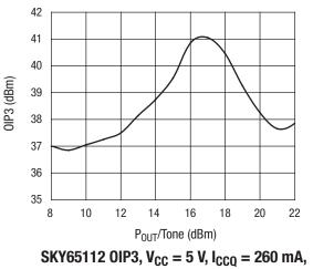
$V_{REF}$  = 5 V, F = 1960 MHz, Tone Spacing = 1 MHz
