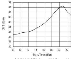
SKY65112 OIP3, V<sub>CC</sub> = 5 V, V<sub>REF</sub> = 5 V, I<sub>CCQ</sub> = 260 mA, F = 450 MHz, Tone Spacing = 1 MHz
