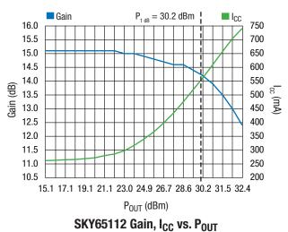
$V_{CC} = 5 \text{ V}, V_{REF} = 5 \text{ V}, I_{CCO} = 260 \text{ mA}, F = 1960 \text{ MHz}$
