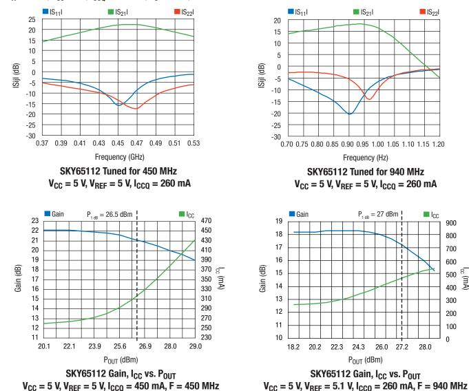
T<sub>A</sub> = 25 °C, V<sub>CC</sub> = 5 V, I<sub>CCQ</sub> = 260 mA, Z<sub>0</sub> = 50  $\Omega$ , unless otherwise noted
