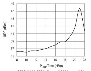
SKY65112 OIP3, V<sub>CC</sub> = 5 V, V<sub>REF</sub> = 5 V, I<sub>CCQ</sub> = 260 mA, F = 2140 MHz, Tone Spacing = 1 MHz
