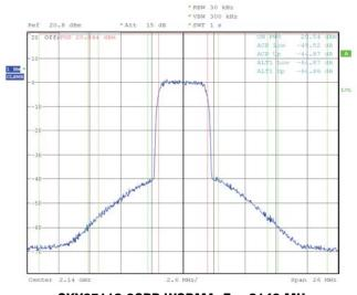
SKY65112 3GPP WCDMA, F = 2140 MHz QPSK 45° Offset, Filter Root Cosine, Roll-off Factor 0.22, Symbol Rate 3.84 Msym/s  $V_{CC} = 5 V$ ,  $V_{REF} = 5 V$ ,  $I_{CCQ} = 260 \text{ mA}$ ,
