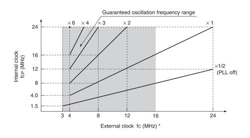
\*: When using the oscillation circuit, the maximum oscillation clock frequency is 16 MHz.
