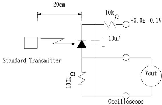
Fig.-3 Measuring System
