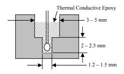
Figure 2 Section View of the 2 Stage Hole
