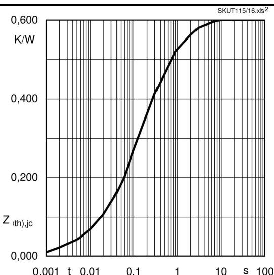
Fig. 2 Transient thermal impedance vs. time
