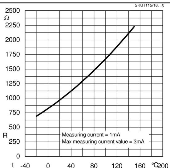
Fig. 6 Temperature sensor characteristic
