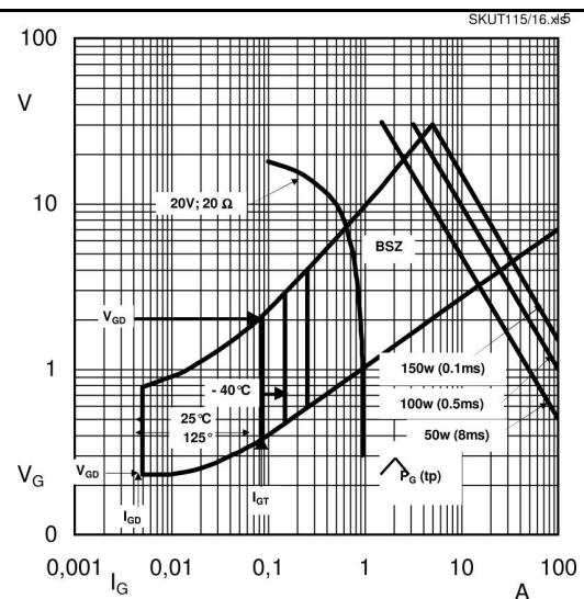
Fig. 5 Gate trigger characteristic
