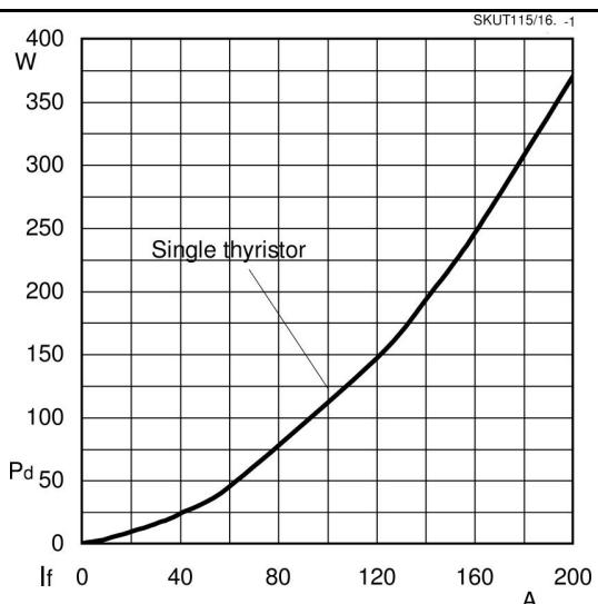
Fig. 1 Power dissipation vs. r.m.s. output current
