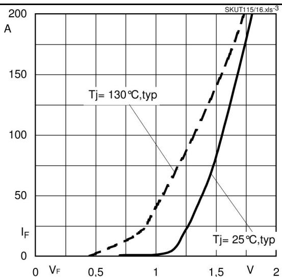
Fig. 3 Forward characteristic of a single thyristor
