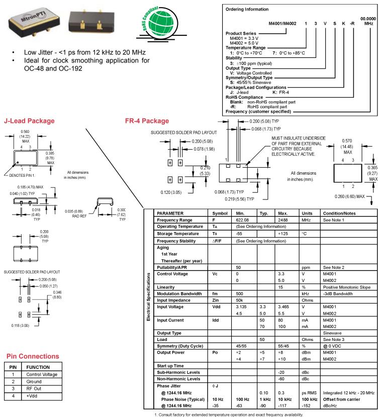
APR specification inclusive of initial calibration, deviation over temperature, shock, vibration, supply voltage, and aging
