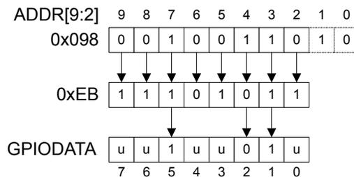
During a read, if the address bit associated with the data bit is set to 1, the value is read. If the address bit associated with the data bit is set to 0, it is read as a zero, regardless of its actual value. For example, reading address GPIODATA + 0x0C4 yields as shown in Figure 9-2 on page 161.
