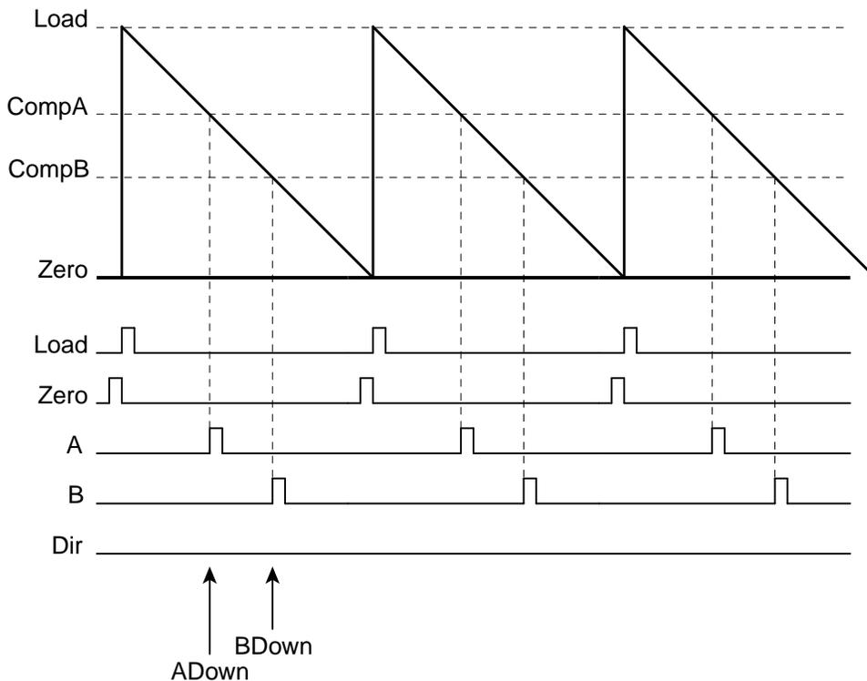
**Figure 18-3. PWM Count-Up/Down Mode**
