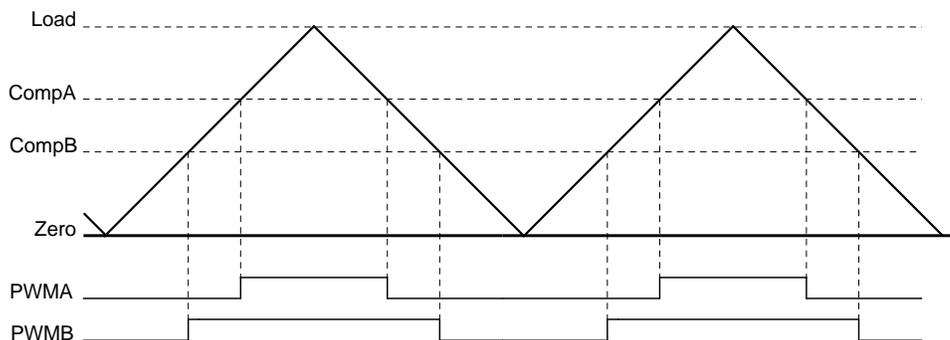
In this example, the first generator is set to drive High on match A up, drive Low on match A down, and ignore the other four events. The second generator is set to drive High on match B up, drive Low on match B down, and ignore the other four events. Changing the value of comparator A
