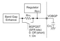
$R_{\text{FIL}}$  is about 100k $\Omega$  and the recommend  $C_{\text{FIL}}$  is 10 $\mu\text{F}.$
