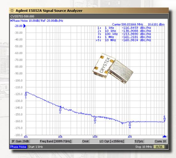
Model CVS575S-500 is a 500MHz voltage-controlled SAW (surface acoustic wave) oscillator (VCSO). SAW crystal technology provides low-noise and low-jitter performance with true sinewave output. Features include -135dBc/Hz phase noise at 10kHz offset, 3.3V input voltage, -20 to +70C operating temperature, and 5x7.5 mm SMT package. The oscillator has no sub-harmonic and the second harmonic is typically -14dBc.
