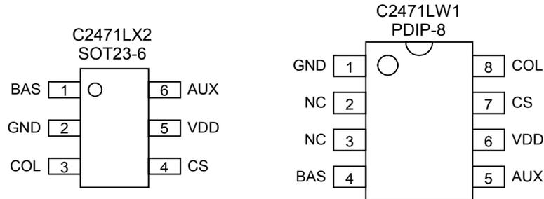
Figure 2: C2471 Pin Assignment
