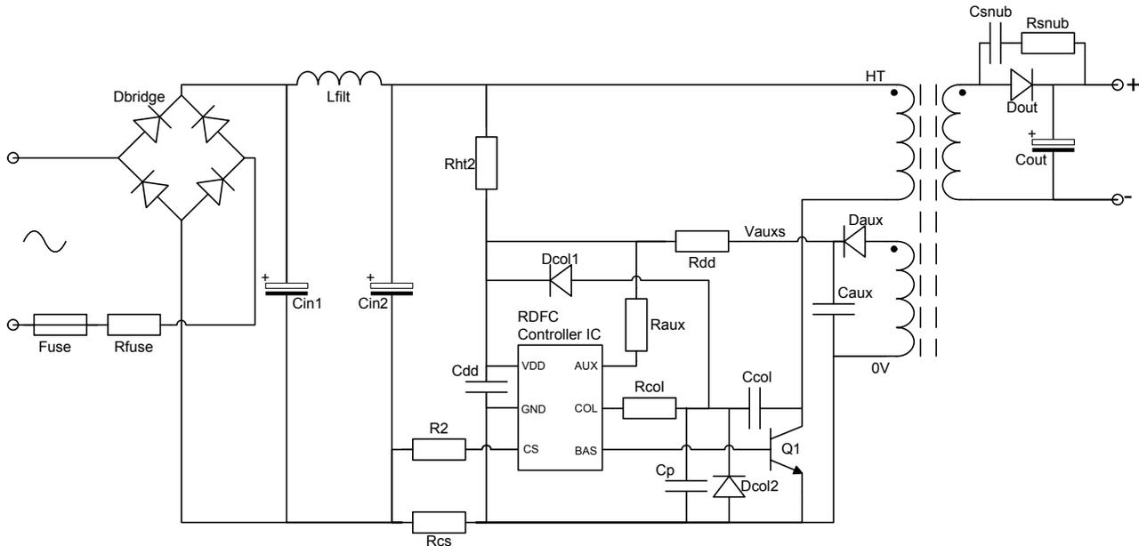
Figure 3: Typical Low Power RDFC Application Schematic
