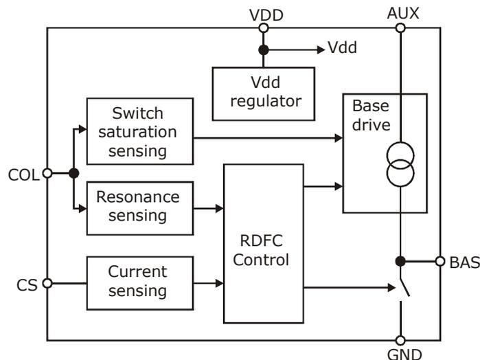
Figure 1: Block Diagram of the C2471 Controller ICs
