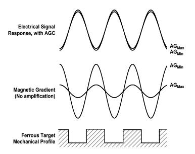
Automatic Gain Control (AGC). The AGC function corrects for variances in the air gap. Differences in the air gap affect the magnetic gradient, but AGC prevents that from affecting device performance.
