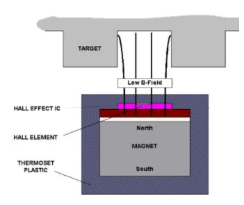
Sensing technology. As the target moves by the sensor, there is a change in the magnetic flux density, B, which is measured in gauss (G). The left panel shows the effect of a tooth opposite the sensor, a higher B. The right panel shows the effect of a valley, a lower B.
