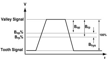
Switch Points. The ATS672 design minimizes hysteresis, B<sub>hvs</sub>.
