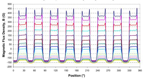
Magnetic Flux Density, B, Versus Air Gap 8X Reference Target Using LSB Package
