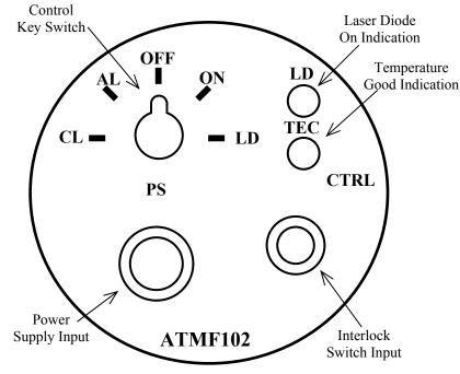
Figure 4 Back View of the Laser
