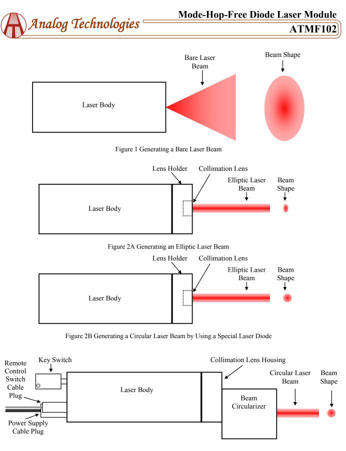
Figure 3 Generating a Circular Laser Beam
