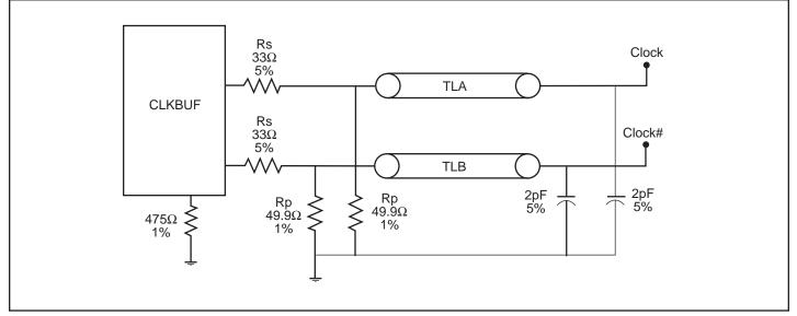
Figure 2. Configuration test load board termination
