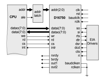
Typical D16750 and processor connection is shown in figure above.
