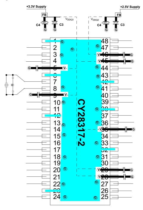
**©** = VIA to GND plane layer **V** = VIA to respective supply plane layer **Note**: Each supply plane or strip should have a ferrite bead and capacitors
