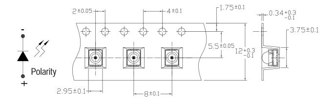
Note: The tolerances unless mentioned is ±0.1mm Unit = mm
