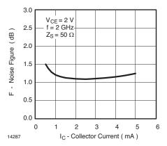
Figure 4. Noise Figure vs. Collector Current
