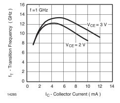
Figure 2. Transition Frequency vs. Collector Current
