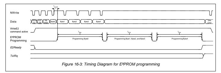
The following diagram shows programming of 5 bytes into the E<sup>2</sup>PROM:
