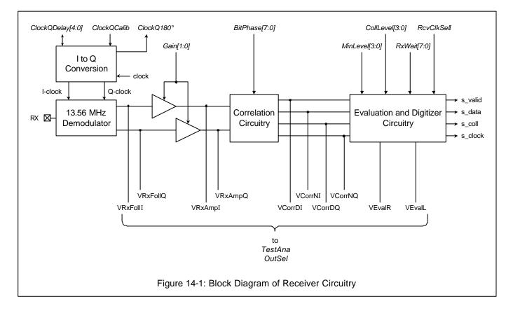
The user may observe the signal on its way through the receiver as shown in the block diagram above. One signal at a time may be routed to pin AUX using the *TestAnaSelect-Register* as described in 18.3.
