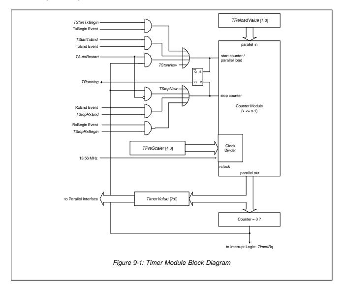
The timer unit is designed in a way, that several events in combination with enabling flags start or stop the counter. For example, setting the bit *TstartTxEnd* to 1 enables to control the receiving of data using the timer unit. In addition the first received bit is indicated by *TxEndEvent*. This combination starts the counter at the defined *TReloadValue*.
