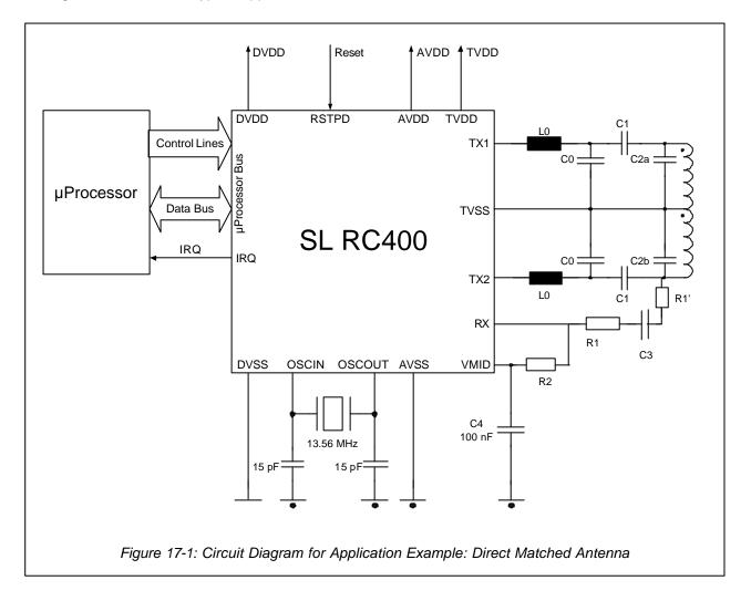
The matching circuit consists of an EMC low pass filter, a receiving circuit, an antenna matching circuit and the antenna itself.
