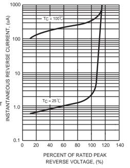
FIG. 2 - TYPICAL REVERSE CHARACTERISTICS
