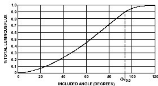
Figure 5.2 Percent total flux vs. included angle for an HPWA-Mx00 LED.
