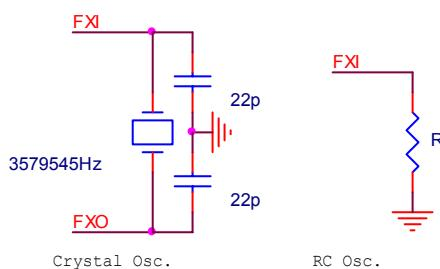
The RC oscillator has a built-in capacitor. An external resistor is needed to connect from FXI to GND to determine the oscillation frequency. The capacitance of internal RC oscillator is selected by mask option MO\_RCAP[2..0].
