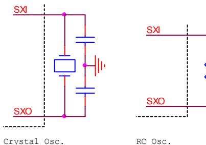
With two clock sources available, the system can switch among operation modes of Fast, Slow, Idle, and Sleep modes by the setting of OP1 and OP2 registers as shown in tables below to suit the needs of application such as power saving, etc.
