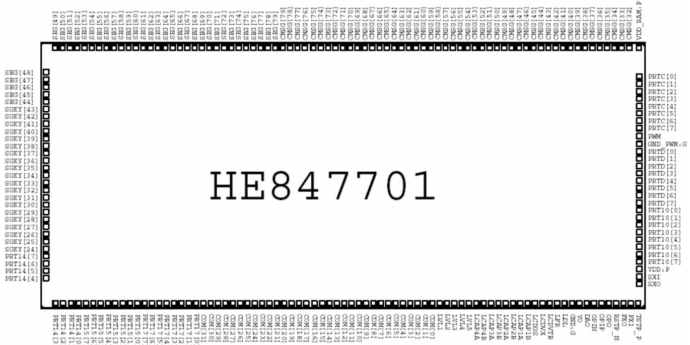
Die Size: X= 9460  $\mu\text{m}$ , Y=4150  $\mu\text{m}$ , and substrate is connected to GND.
