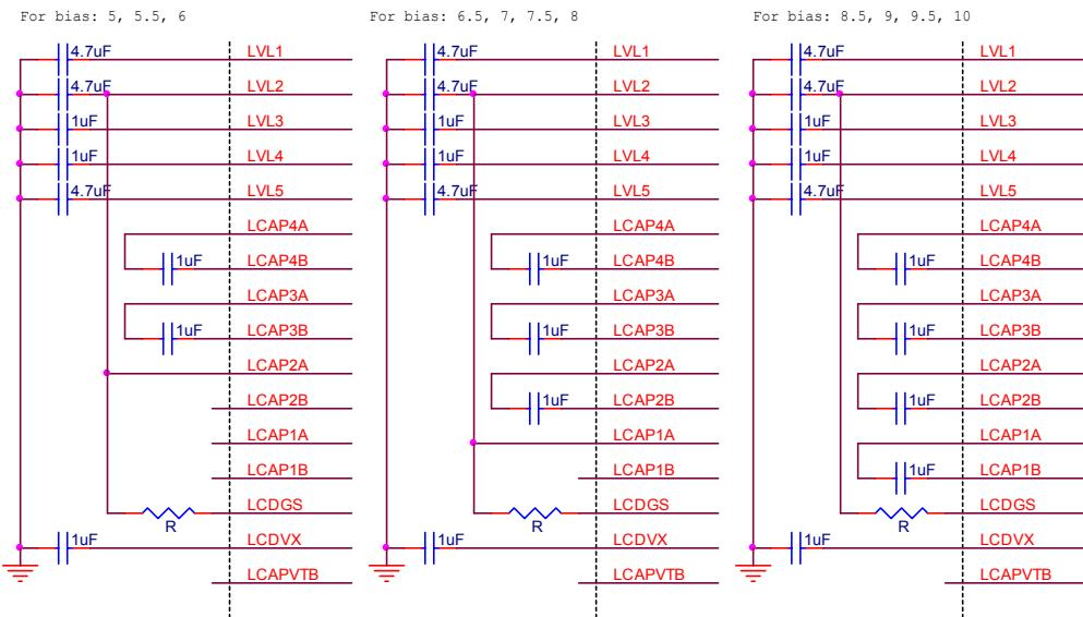
Different duties require different bias settings. There is some theoretical correspondence between the Duty and Bias Setting. However, it is better to use it as starting point and adjust it with real LCD panel connected to it to determine the final setting. The theoretic relationship between the duty and bias setting as following:
