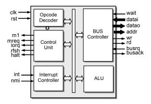
**Bus Controller** –Data Memory & SFR's (Special Function Register) interface controls access into the program and data memories and special registers. It contains Program Counter (PC), Stack Pointer (SP) register, Index registers and related logic.
