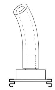
Fig. 10: connection to pressure port
