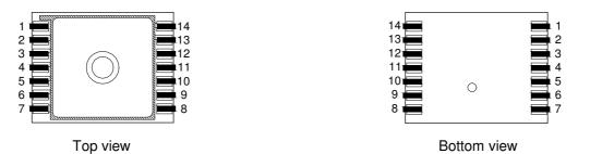
Fig. 2: Pin configuration of MS5536-PJU, MS5536-NJU
