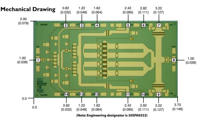
Units: millimeters (inches) Bond pad dimensions are shown to center of bond pad. Thickness: 0.110 + -0.010 (0.0043 + -0.0004), Backside is ground, Bond Pad/Backside Metallization: Gold All DC Bond Pads are  $0.100 \times 0.100 (0.004 \times 0.004)$ . All RF Bond Pads are  $0.100 \times 0.200 (0.004 \times 0.008)$  Bond pad centers are approximately 0.109 (0.004) from the edge of the chip. Dicing tolerance: +/-0.005 (+/-0.0002). Approximate weight: 4.588 mg.
