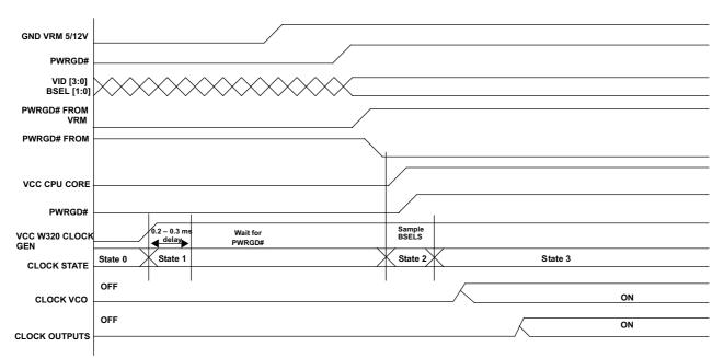
Figure 3. CPU Power AFTER Clock Power
