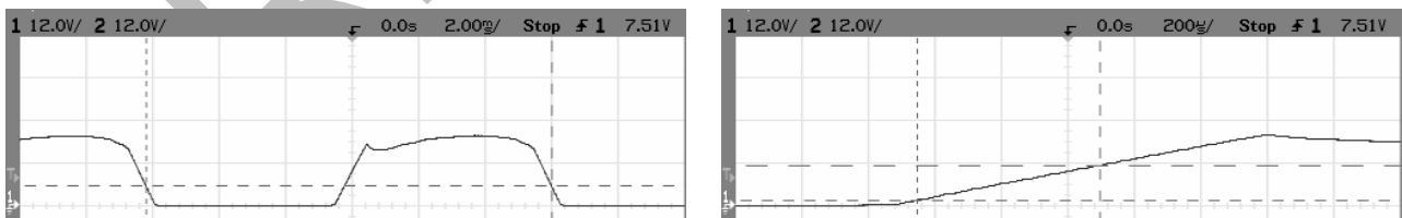
(a) – General view (b) – Enlarged view on output switching Figure 3 – Output voltage with long output slope duration ( R_{SLOPE} = 500k )
