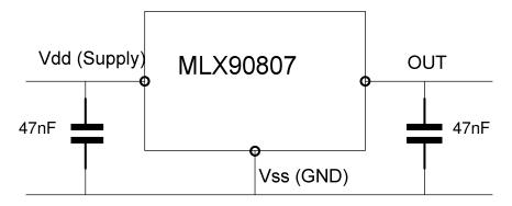
Very few off-chip components are needed (only 2 decoupling capacitors, <u>not higher than 100 nF</u>). Only 3 pins are used (Vdd, Vss, Out), see pad layout drawing in paragraph 9. Calibration and Programming is made through the OUT pin.
