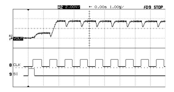
In the first figure, one can see clearly a first SI pulse, followed by 133 CLK pulses. After the selected integration time, a next SI pulse is generated, again accompanied with 133 CLK pulses. Note that the CLK pulses have stopped. During the CLK pulses, the pixel values of the former integration time are clocked out. This screenshot repeats itself continously for every new scan.
