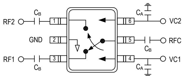
DC blocking capacitors  $C_B = 8\text{pF}$  and by-pass capacitors  $C_A=8\text{pF}$  are required on all RF ports and control lines.
