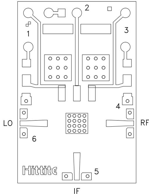
The grounded Co-Planar Wave Guide (CPWG) PCB input/output transitions allow use of Ground-Signal-Ground (GSG) probes for testing. Suggested probe pitch is 400  $\mu$ m (16 mils). Alternatively, the board can be mounted in a metal housing with 2.4 mm coaxial connectors.
