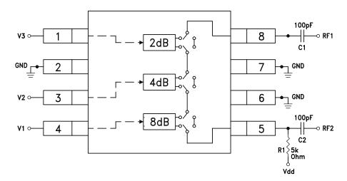
DC blocking capacitors C1 & C2 are required on RF1 & RF2. Choose C1 = C2 = 100 ~ 300 pF to allow lowest customer specific frequency to pass with minimal loss. R1 = 5K Ohm is required to supply voltage to the circuit throught either PIN 5 or PIN 8.
